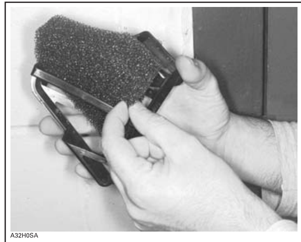
Removal of filter from its grill
