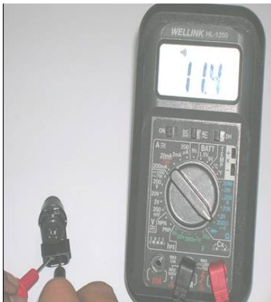
Injector resistance confirmation
