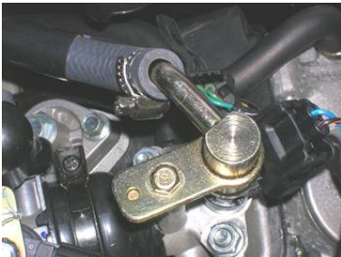
Fuel pressure measurement demolition - injector
