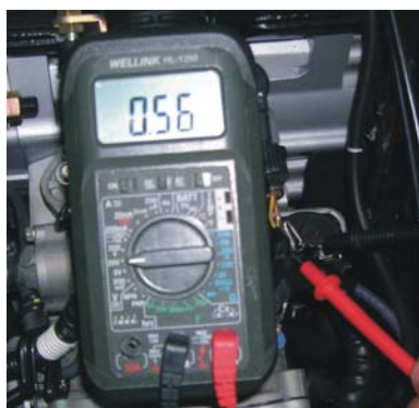
Throttle output signal measurement - full closed
