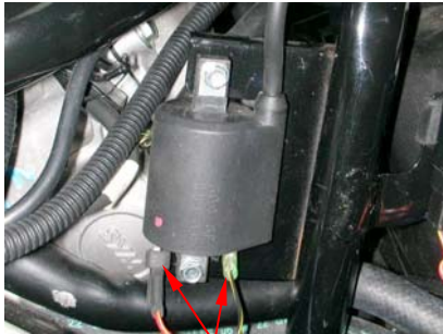
First circuit coil resistance measurement
