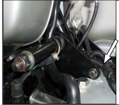
MAGNETO WIRES ROUTING
