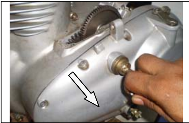
Application :To remove Crank case LH cover
