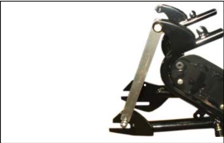
Application : Alignment of Swing Arm while tightening
