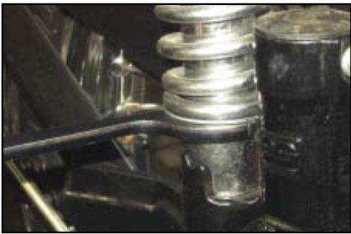
Application :To adjust gas filled shock absorber
