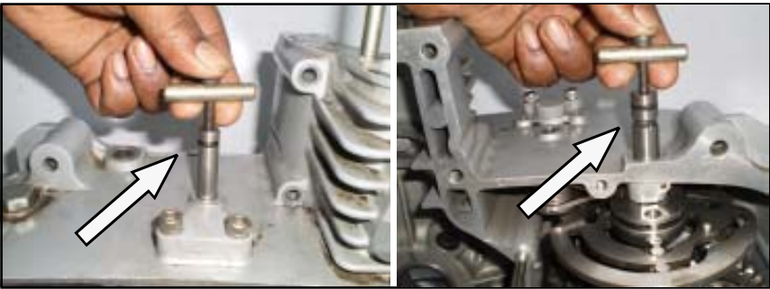
Application : To remove Gear Rocker Shaft top pivot pin and Gear Cam Plate pivot pin.
