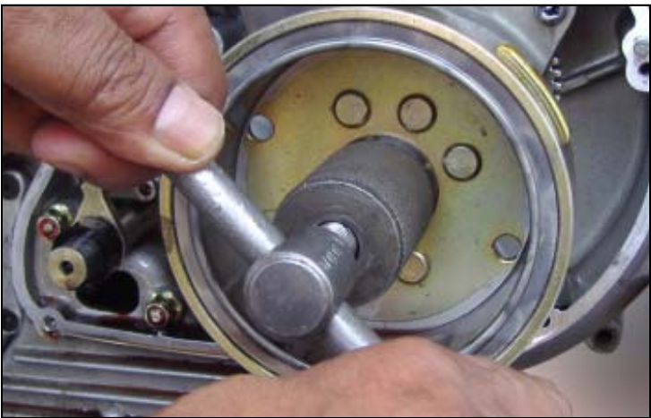
Application : Removal of magneto assembly
