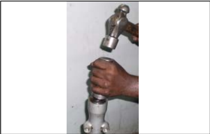
Application : Fitment of oil seal in front fork bottom tube
