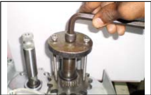
Application : To remove front drive sprocket from Sleeve Gear.
