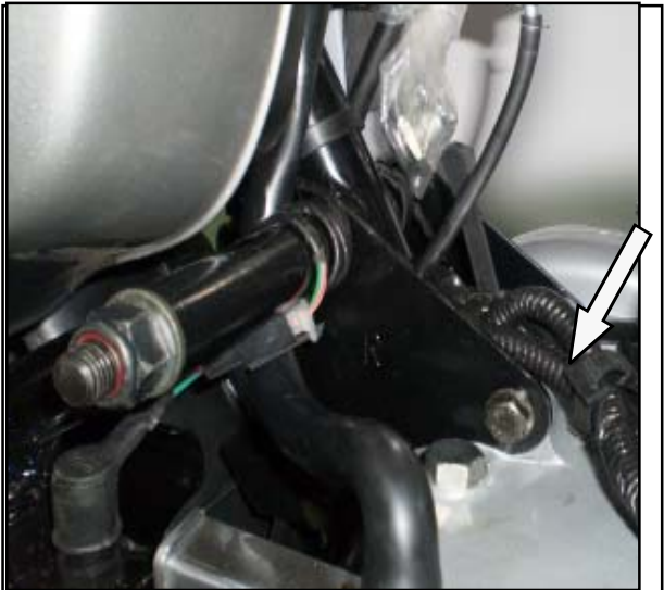
MAGNETO WIRES ROUTING
