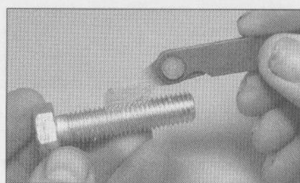
2.12 Using a thread gauge to measure pitch
