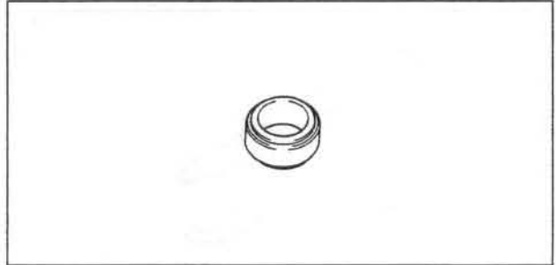
Head Pipe Outer Race Press Shaft: 57001-1075
