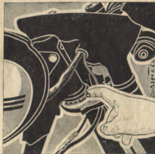
Fig. 46 - Lubricating the steering head ball bearing
