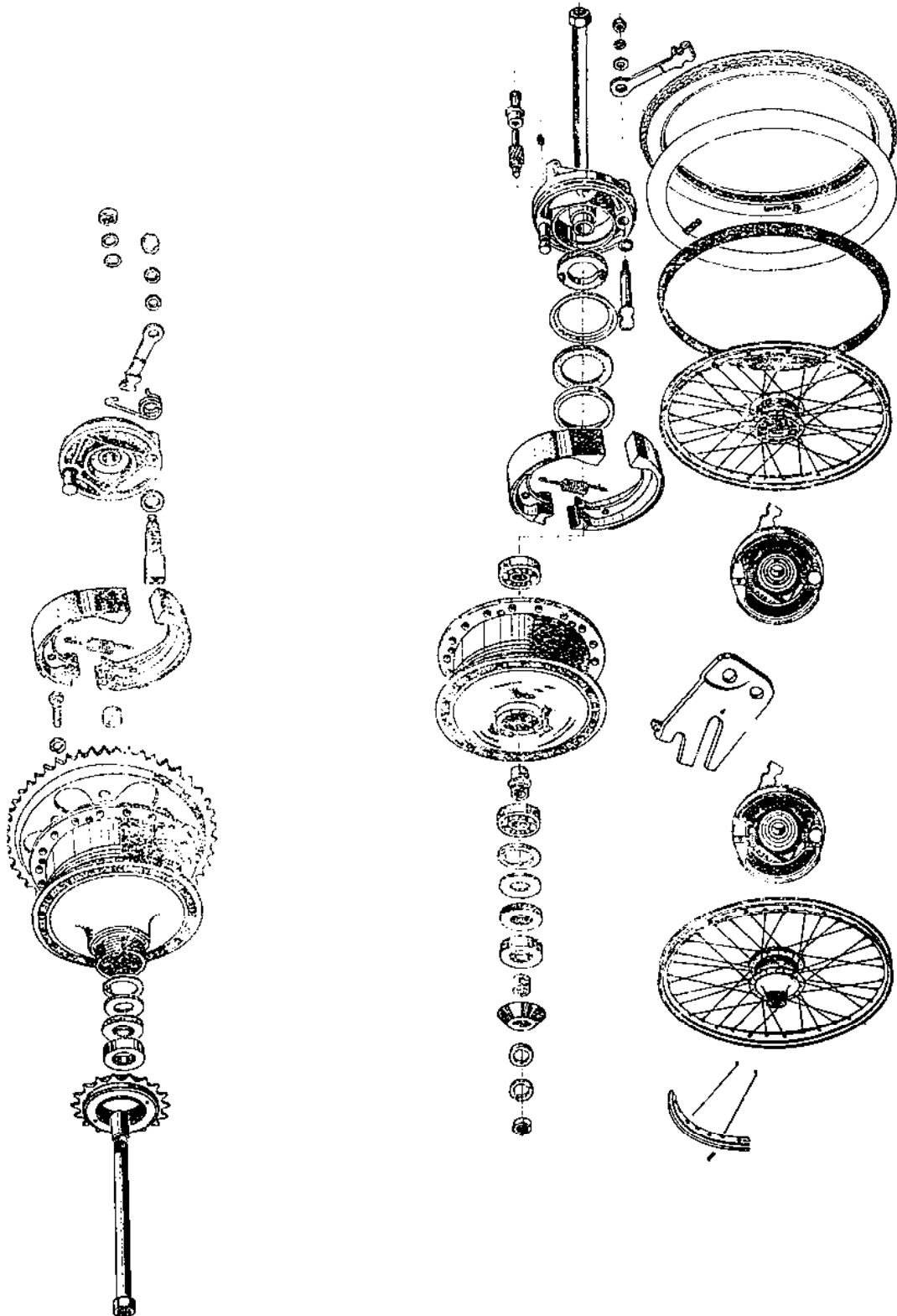
Fig. 26 Exploded view of front and rear wheel.
