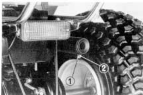
(1) Spark arrester bolts (2) Sealing washer
