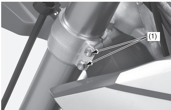
(1) fork bridge lower pinch bolts
