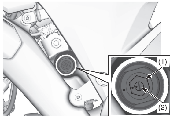
(1) high speed compression damping adjuster (2) low speed compression damping adjuster
