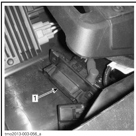
1. Auxiliary fuse box
