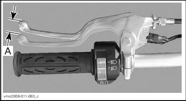
CLUTCH LEVER — NOMINAL FREE PLAY A. 10 to 15 mm (3/8 to 5/8 in)
