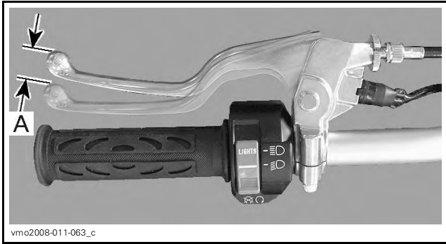
CLUTCH LEVER — PROPER ADJUSTMENT A. 10 to 15 mm (3/8 to 5/8 in)
