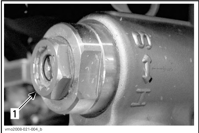
3/4 OF A TURN 1. High speed compression adjuster
