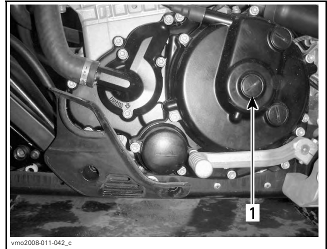
LH SIDE OF ENGINE 1. Access plug
