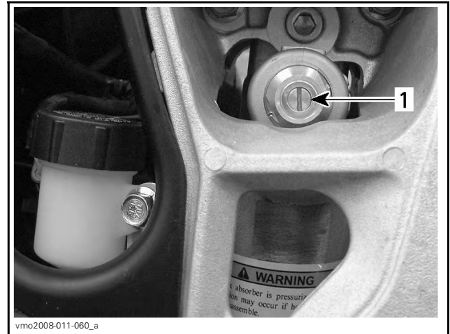
9 CLICKS COUNTERCLOCKWISE 1. Compression damping adjuster
