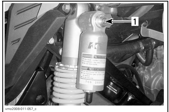
9 CLICKS COUNTERCLOCKWISE 1. Compression adjuster
