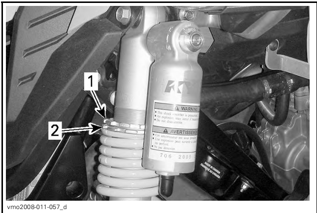
1. Locking ring 2. Adjusting ring
