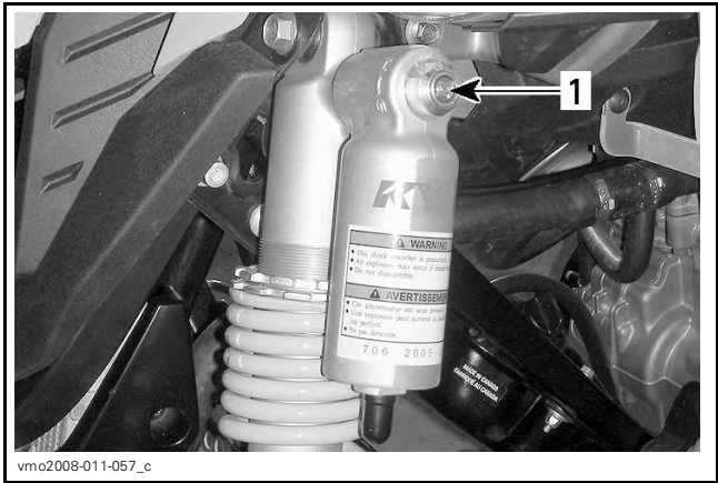
8 CLICKS COUNTERCLOCKWISE 1. Compression adjuster
