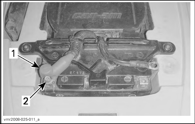
1. Pull out protective boot 2. Disconnect RED (+) battery cable
