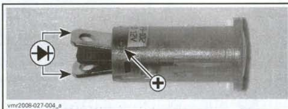
NEUTRAL INDICATOR LIGHT LED TESTING
