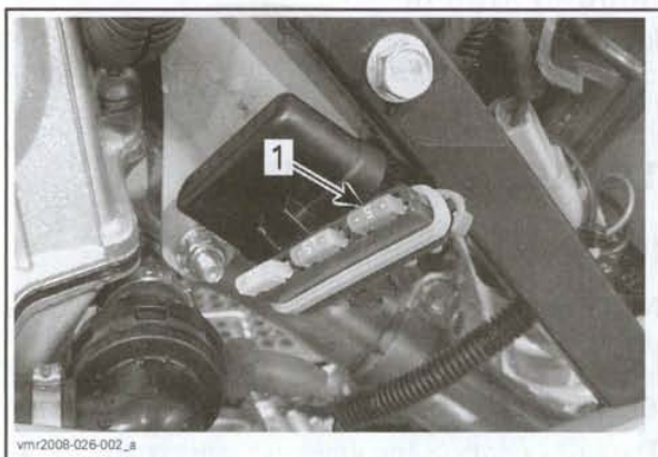
PF1 FUSE HOLDER 1. 5 A ECM fuse
