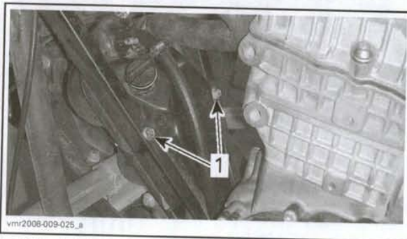
1. Oil tank bolts
