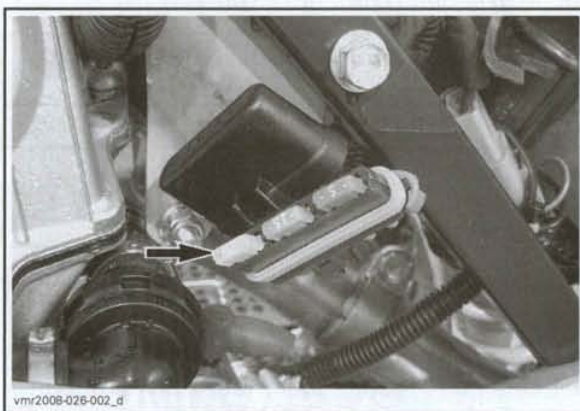
REMOVE 20 A COOLING FAN/ACCESSORIES FUSE
