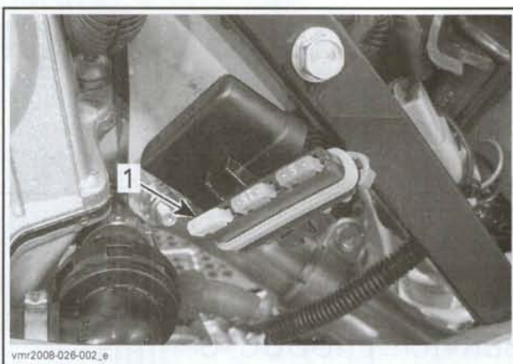
PF1 FUSE HOLDER 1. 20 A cooling fan fuse
