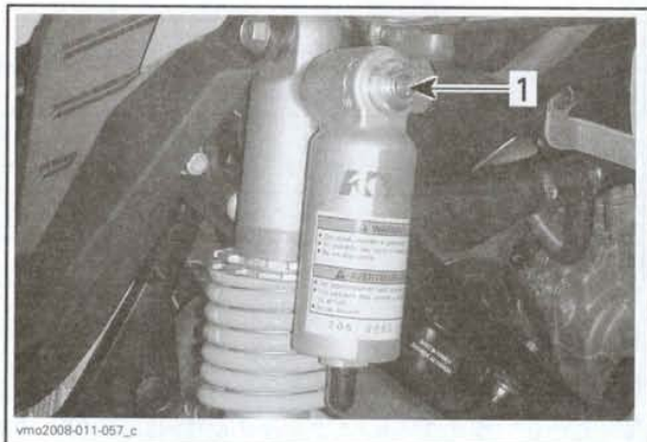
8 CLICKS COUNTERCLOCKWISE 1. Compression adjuster
