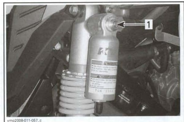
9 CLICKS COUNTERCLOCKWISE 1. Compression adjuster
