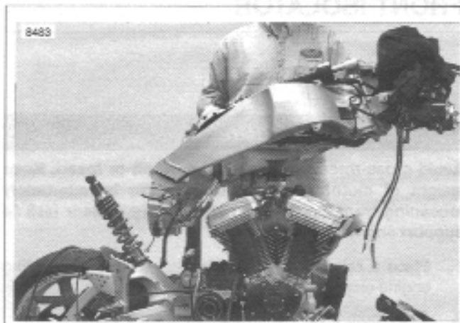
Figure 2-82. Lift Frame Off Motorcycle
