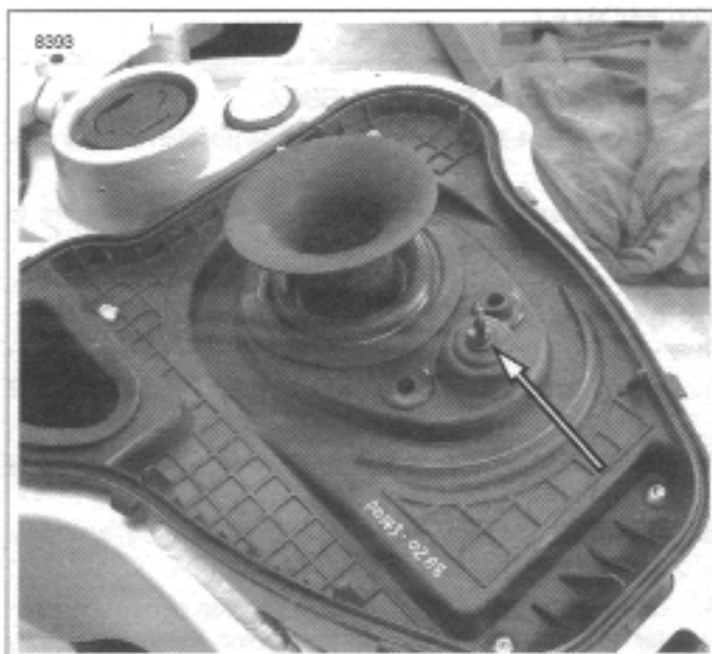
Figure 4-79. Intake Air Temperature Sensor Installed
