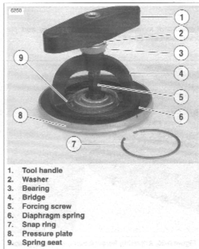
Figure 6-34. Pressure Plate Assembly
