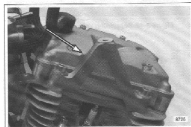
Figure 3-36. Center Tie Bar Mount
