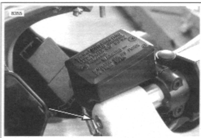
Figure 2-96. Handlebar Clip-on Mounting Fasteners (right clip-on shown)
