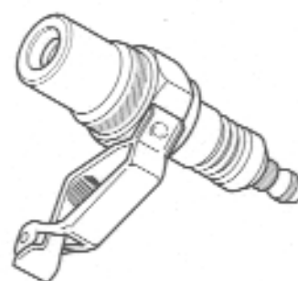
Figure 4-19. Spark Plug Tester (Part No. HD-26792)
