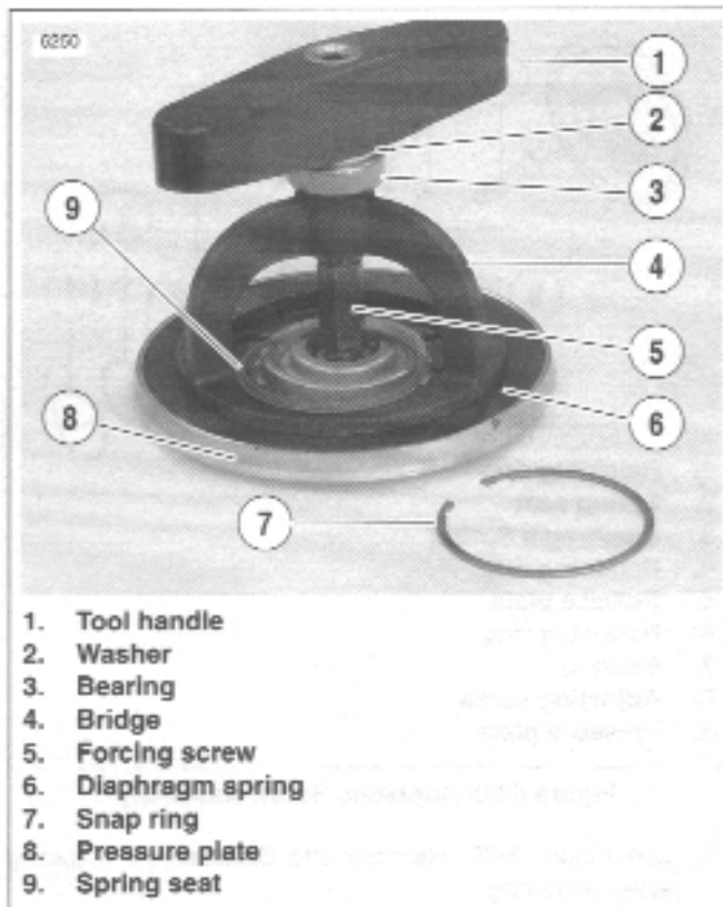
Figure 6-19. Pressure Plate Assembly
