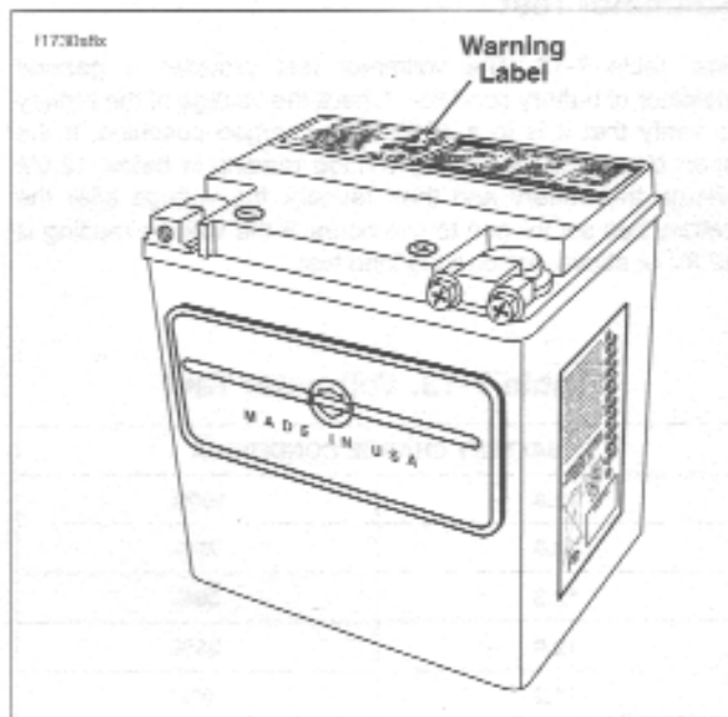
Figure 7-38. Maintenance-Free Battery (Typical)
