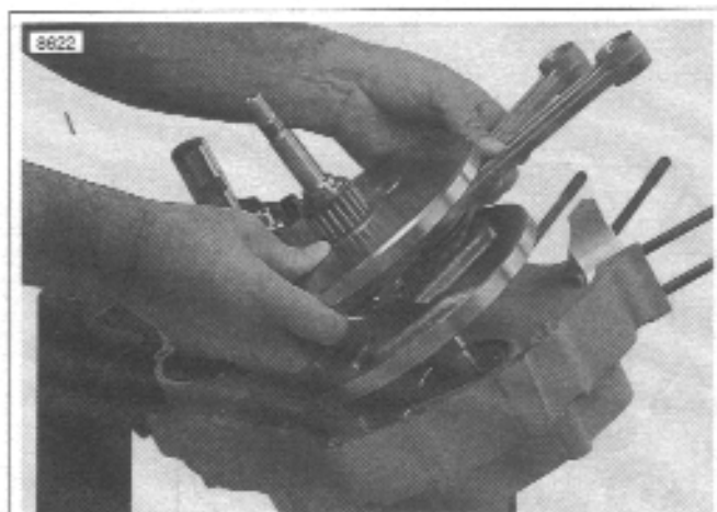
Figure 3-136. Removing Flywheels from Left Crankcase
