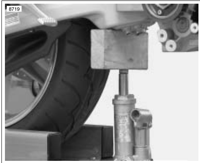
Figure 3-38. Supporting the Swingarm
