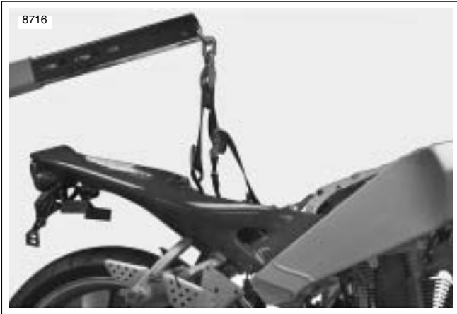
Figure 3-24. Supporting Vehicle for Disassembly (Typical)
