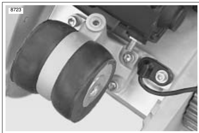
Figure 3-31. Rear Isolator and Mounting Hardware
