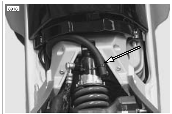
Figure 3-27. Transmission Vent Line
