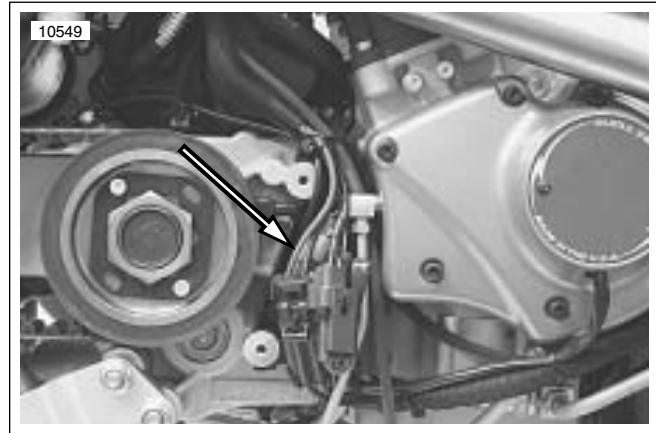
Figure 7-28. Positive Regulator Cable (red wire)
