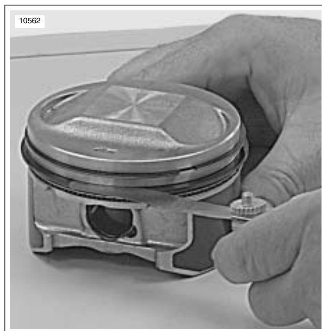
Figure 3-99. Measuring Ring Clearance in Groove
