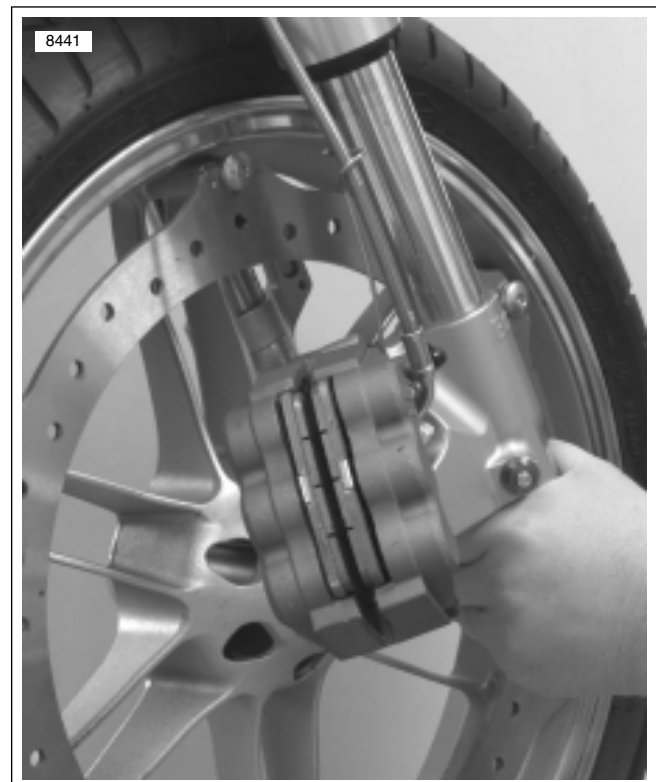
Figure 2-6. Front Wheel Removal
