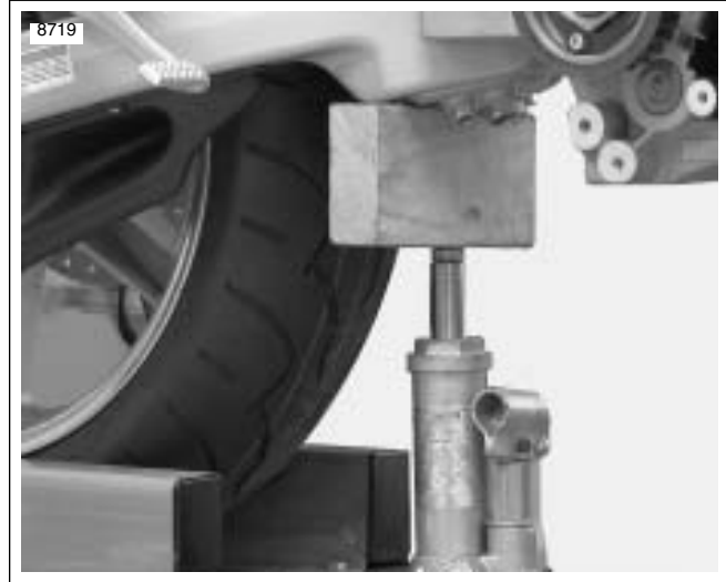
Figure 3-26. Supporting the Swingarm
