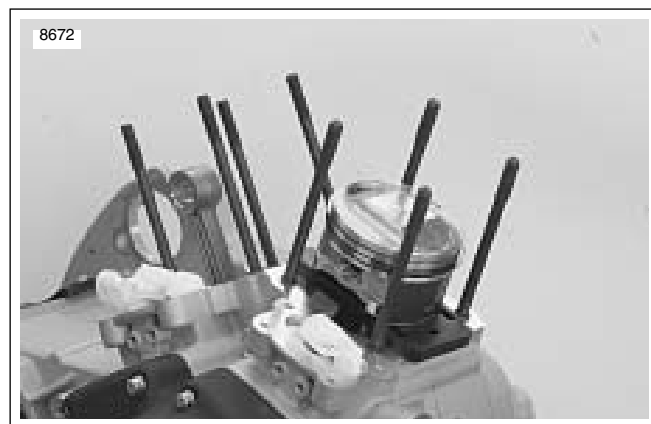
Figure 3-108. Piston Support Plate
