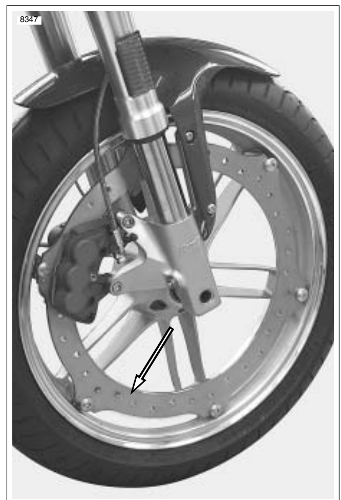
Figure 1-14. Front Brake Rotor
