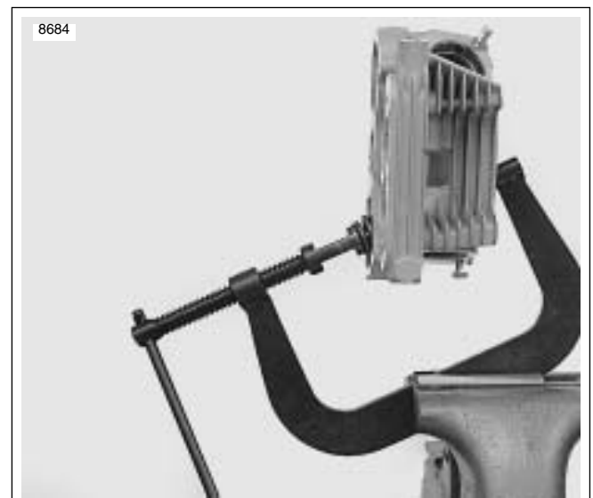
Figure 3-64. Valve Spring Compressor (Part No. HD-34736B)
