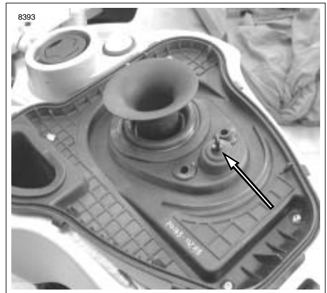
Figure 4-78. Intake Air Temperature Sensor Installed
