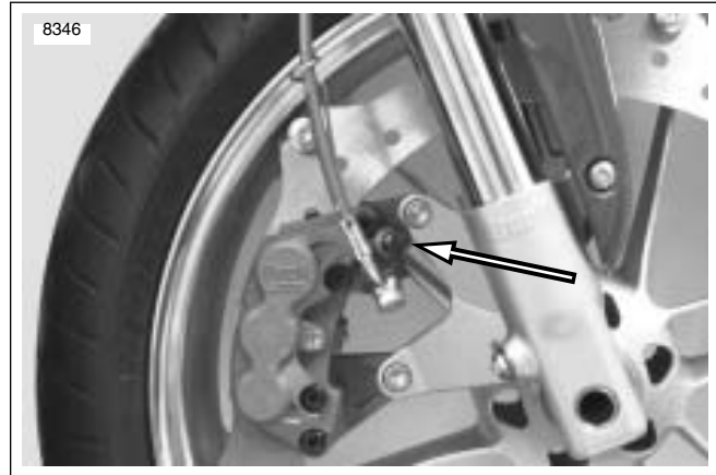
Figure 1-7. Front Caliper Bleeder Valve
