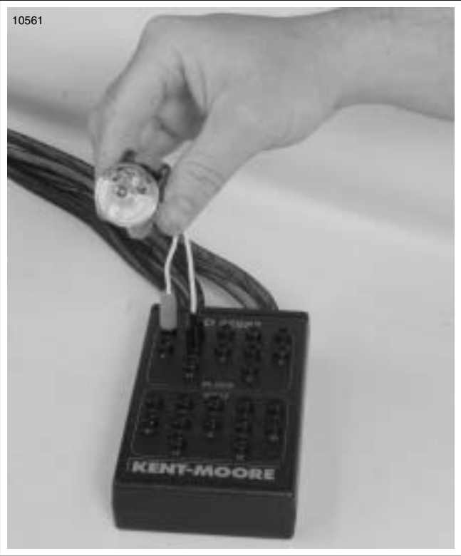
Figure 4-19. Ignition Coil Circuit Test
