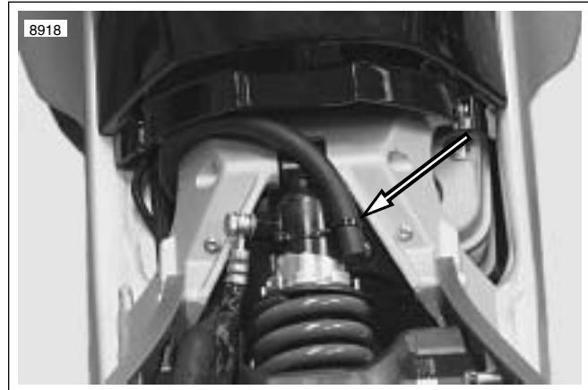
Figure 3-40. Transmission Vent Line
