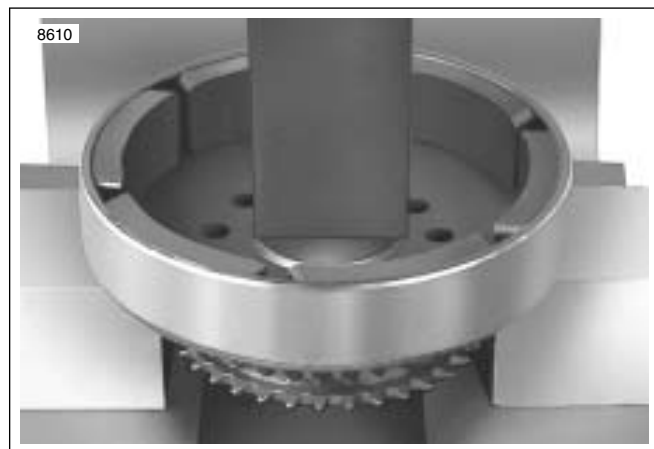
Figure 7-33. Removing Rotor From Sprocket
