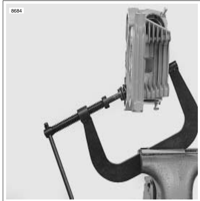
Figure 3-82. Valve Spring Compressor (Part No. HD-34736B)
