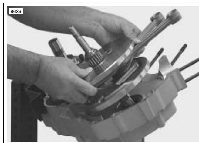
Figure 6-53. Removing Flywheels from Left Case Half
