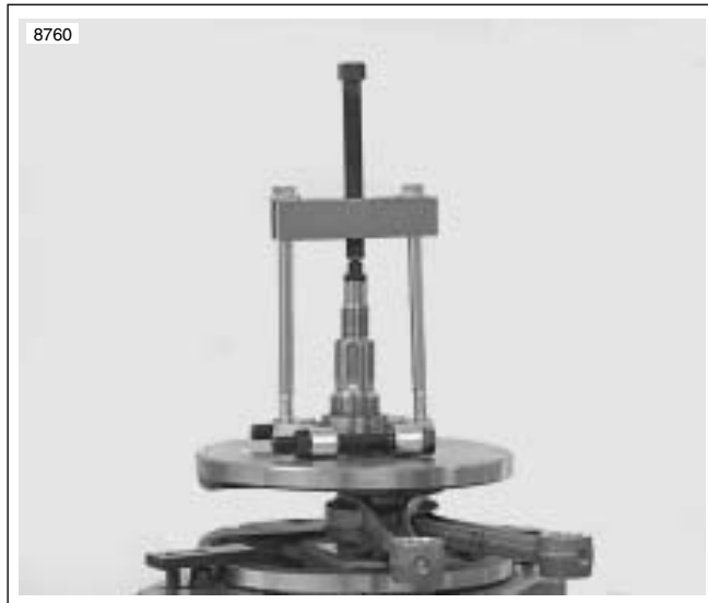
Figure 3-136. Removing Sprocket Shaft Inner Bearing Race
