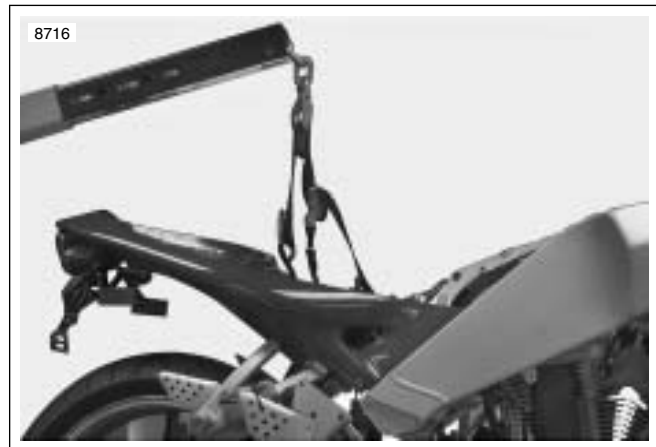
Figure 3-41. Supporting Vehicle for Assembly (Typical)
