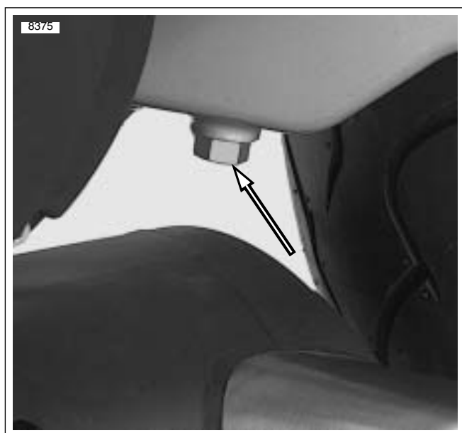
Figure 1-4. Oil Tank Drain Plug
