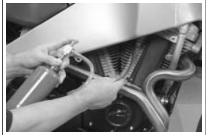
Figure 4-108. Checking for Intake Leak
