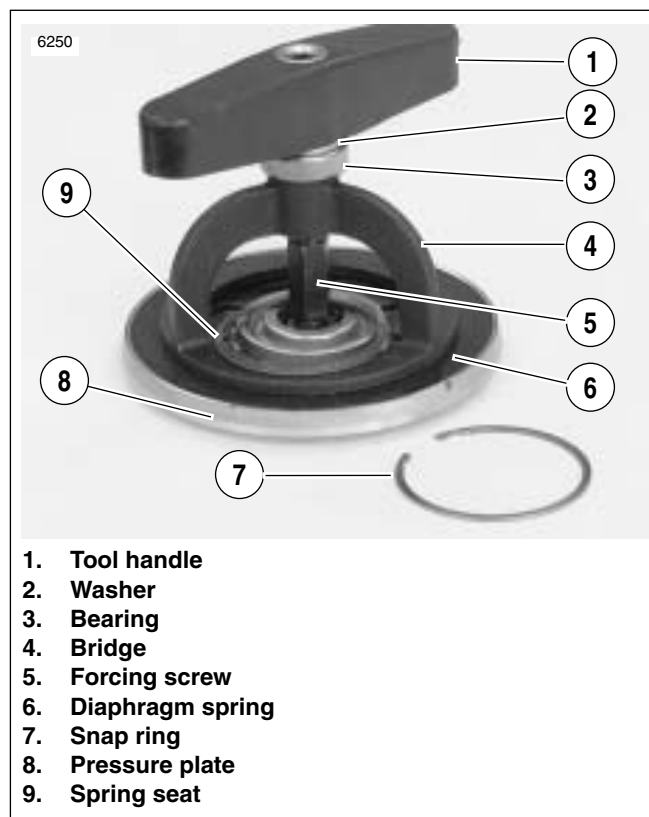
Figure 6-11. Pressure Plate Assembly
