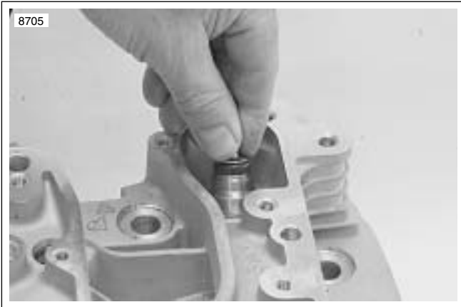
Figure 3-81. Valve Seal and Lower Collar Assembly Installation
