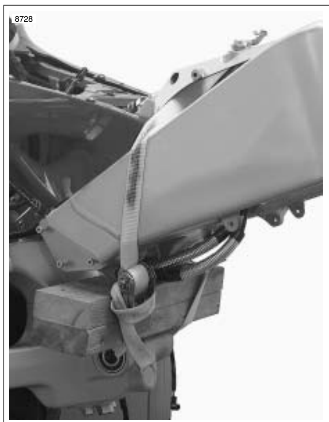
Figure 3-32. Securing Vehicle for Relocation (Typical)
