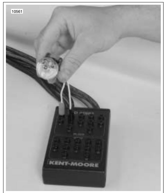
Figure 4-48. Testing Ignition Coil Connectors
