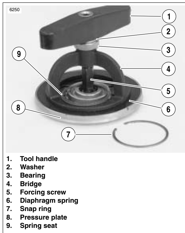
Figure 6-19. Pressure Plate Assembly
