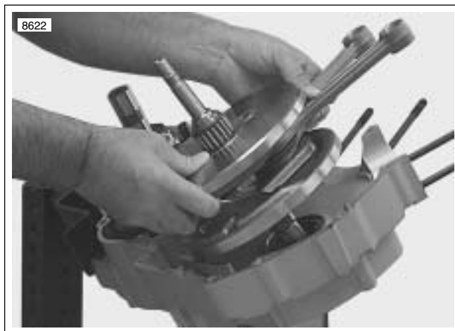
Figure 3-134. Removing Flywheels from Left Crankcase
