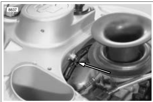
Figure 7-82. Wire Harness Clip
