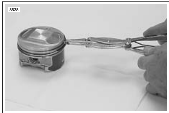
Figure 3-92. Removing Piston Rings
