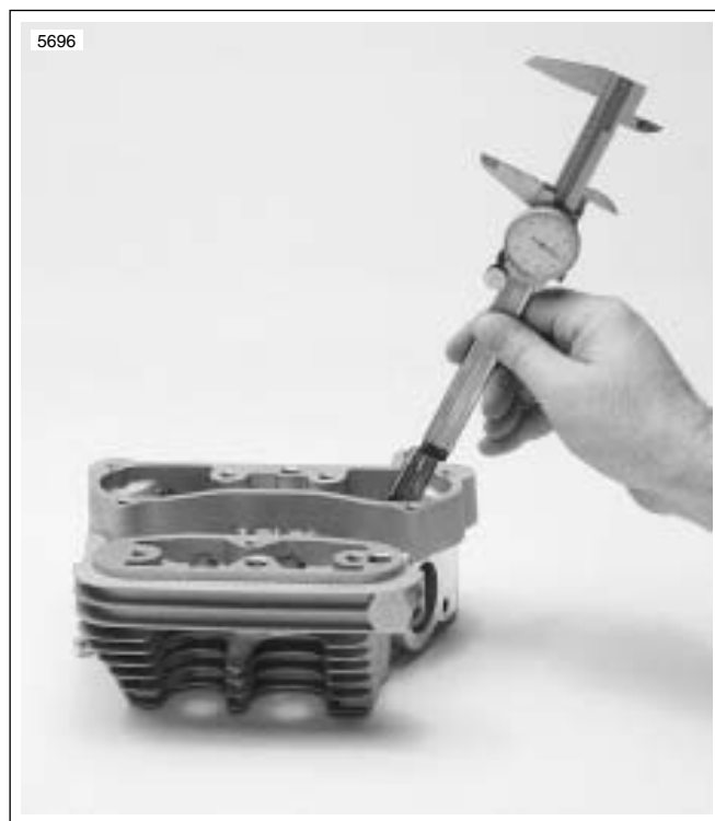
Figure 3-71. Measuring Valve Stem Protrusion
