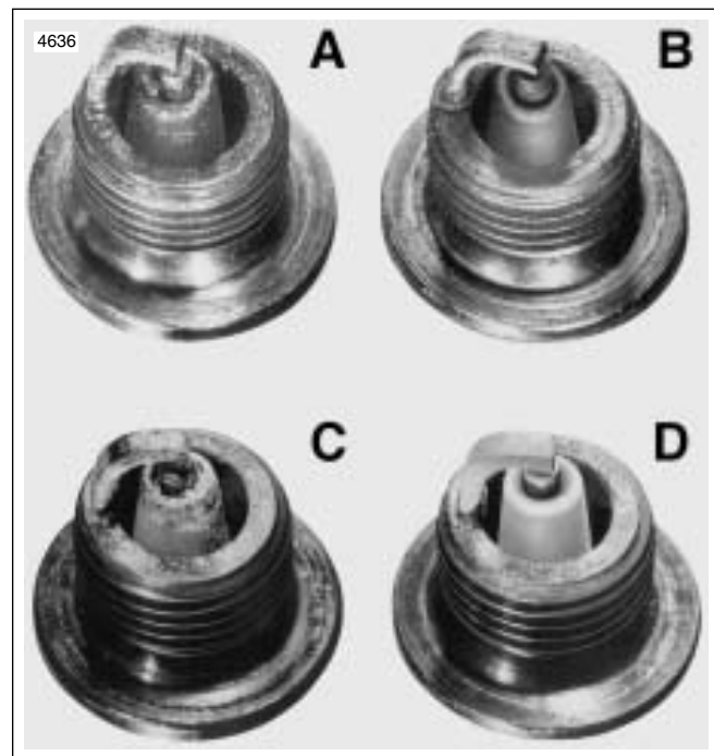
Figure 1-35. Typical Spark Plug Deposits
