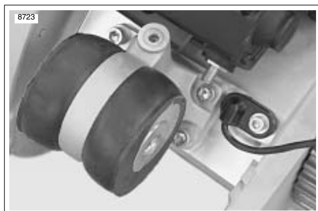
Figure 3-34. Rear Isolator and Mounting Hardware
