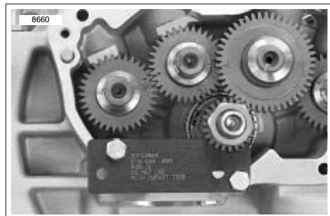
Figure 3-128. Crankshaft Locking Tool (Part No. HD-43984)
