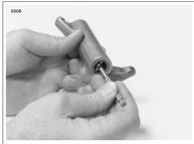
Figure 3-70. Measuring Rocker Arm Bushing Inner Diameter
