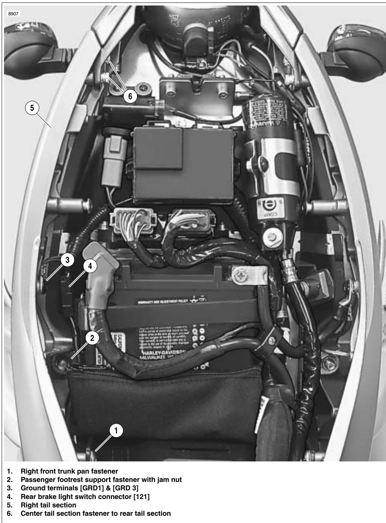
Figure 2-115. Right Side Frame Section
