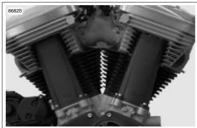
Figure 3-83. Push Rod Locations
