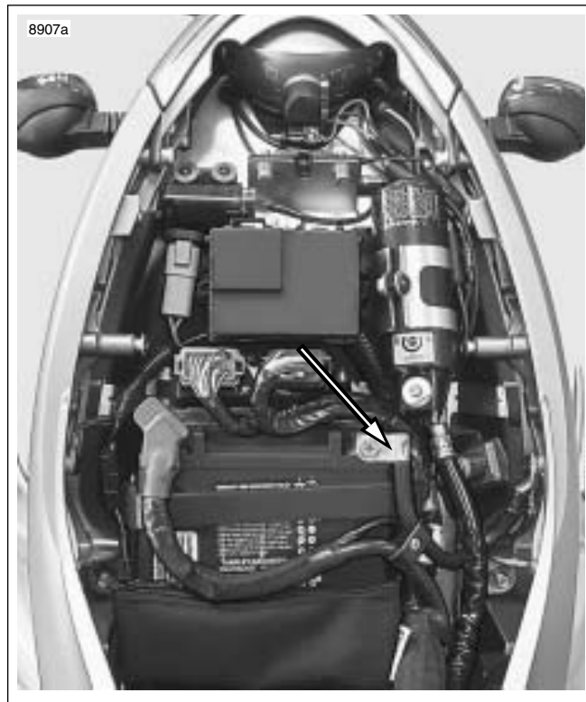
Figure 7-44. Negative Battery Cable
