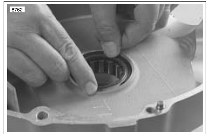
Figure 3-138. Removing Left Main Bearing Retaining Ring
