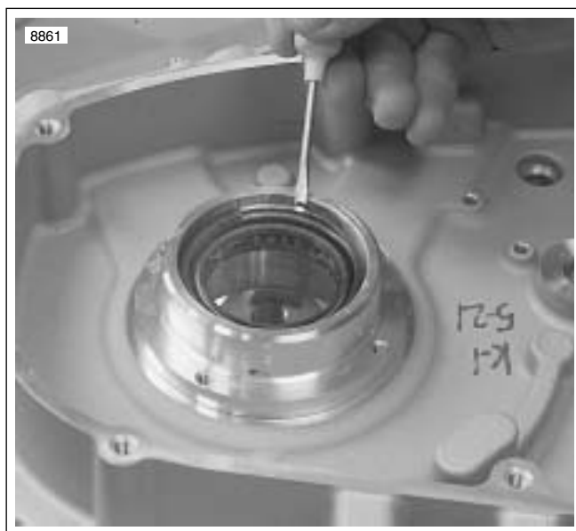
Figure 3-137. Left Main Seal Retaining Ring
