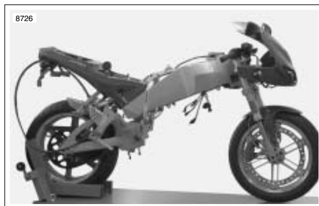
Figure 3-33. Rolling Chassis (Typical)
