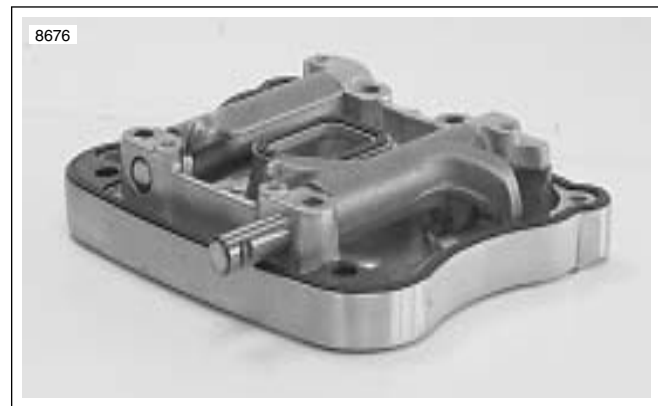
Figure 3-62. Removing Rocker Arm Shafts
