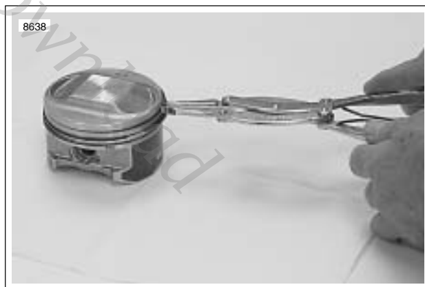
Figure 3-92. Removing Piston Rings
