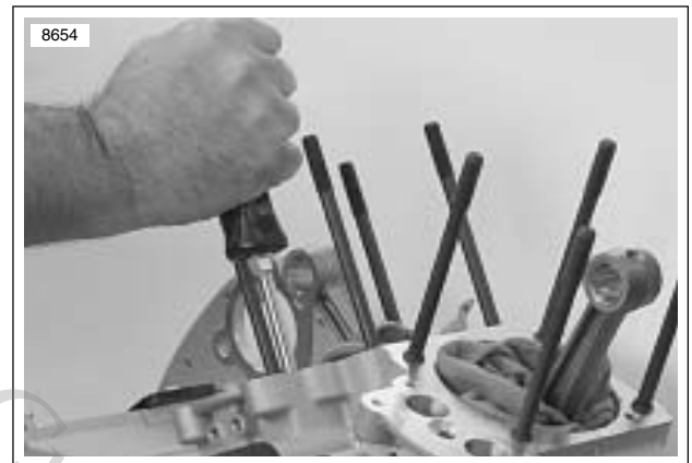
Figure 3-132. Checking Cam Gear End Play
