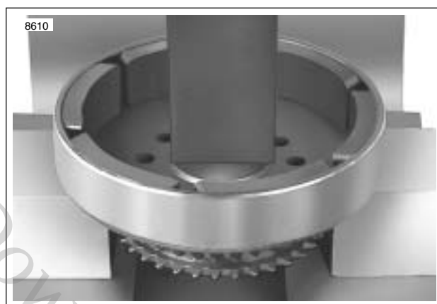
Figure 7-33. Removing Rotor From Sprocket
