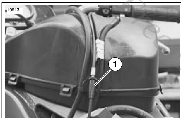
Figure 1-45. Checking For 1/8 in. (3.18) Maximum Free Play In Either Direction For Proper Adjustment
