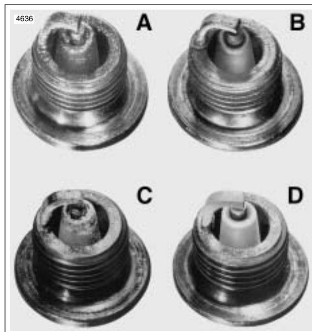
Figure 1-36. Typical Spark Plug Deposits
