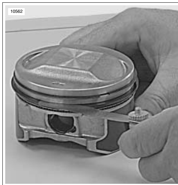
Figure 3-99. Measuring Ring Clearance in Groove
