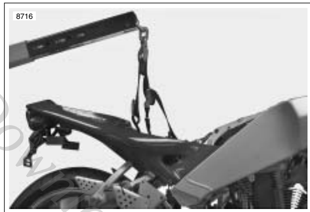
Figure 3-41. Supporting Vehicle for Assembly
