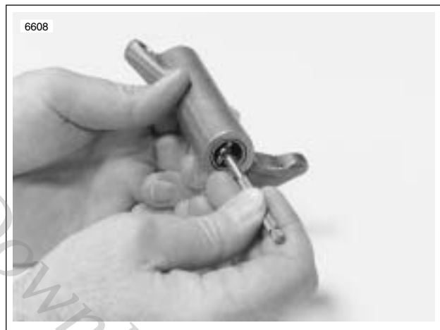
Figure 3-70. Measuring Rocker Arm Bushing Inner Diameter
