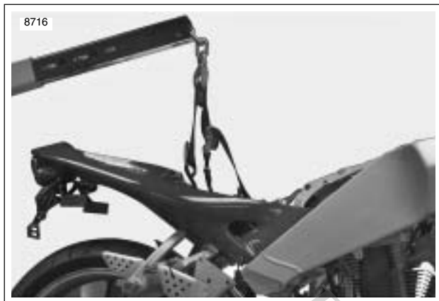
Figure 3-24. Supporting Vehicle for Disassembly
