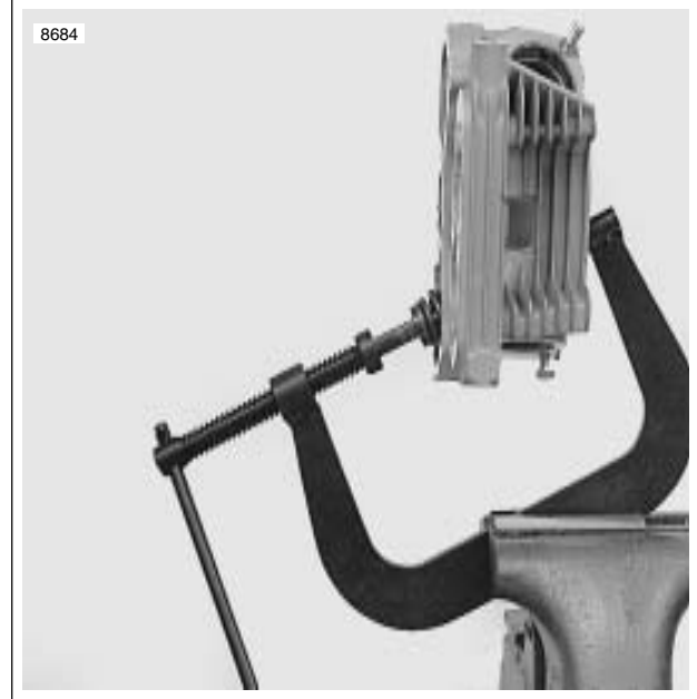
Figure 3-82. Valve Spring Compressor (Part No. HD-34736B)
