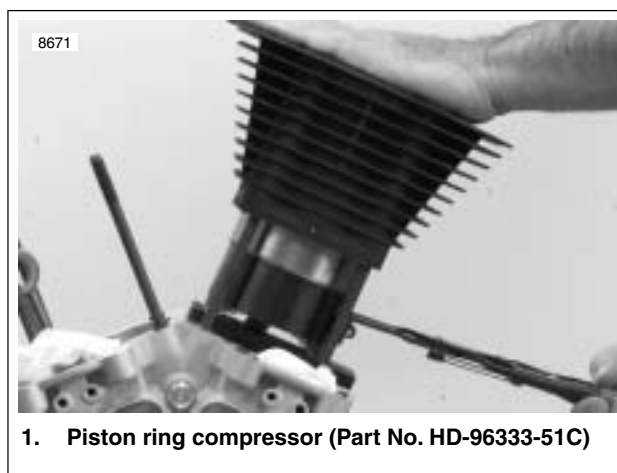
Figure 3-109. Compressing Piston Rings
