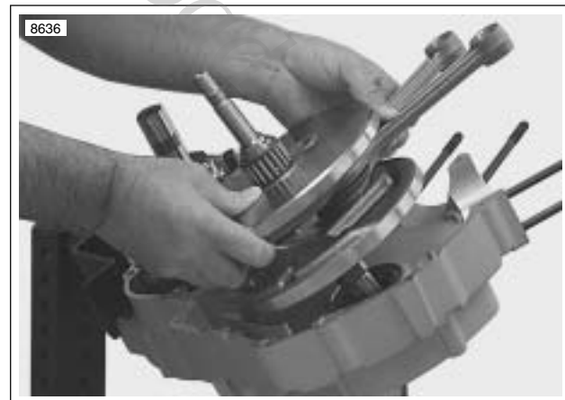
Figure 6-56. Removing Flywheels from Left Case Half
