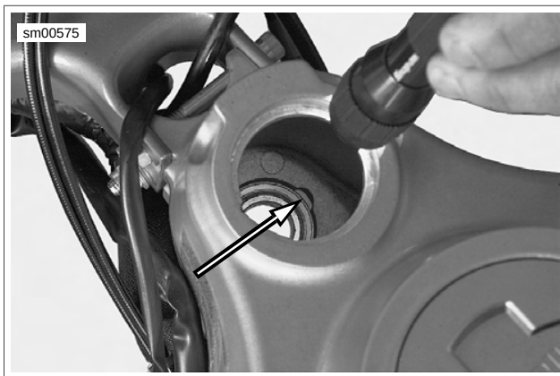
Figure 2-102. Lower Steering Head Bearing Notches (Upper Bearing Removed For Clarity)
