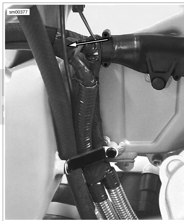
Figure 7-58. Interactive Exhaust Cable Behind Wire Harness Strap and Guide
