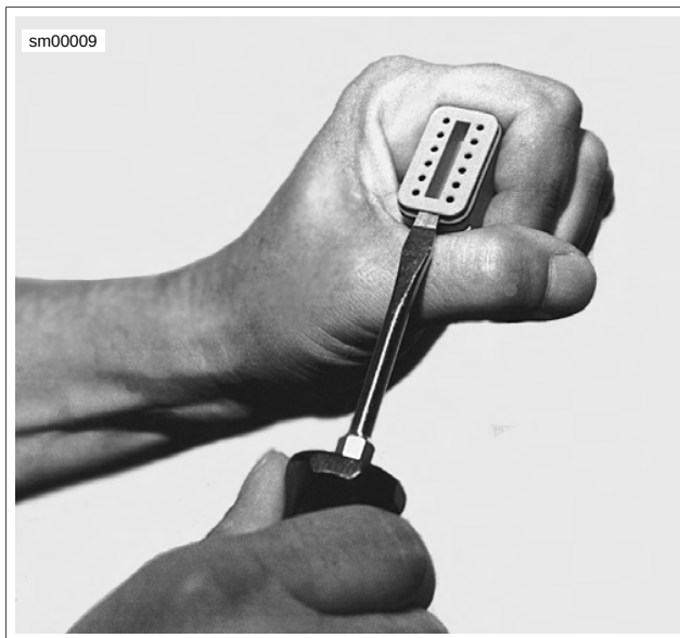
Figure A-15. Deutsch Connector: Remove Secondary Locking Wedge
