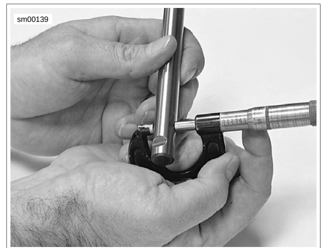
Figure 3-51. Measuring Rocker Arm Shaft Diameter (Rocker Arm Bushing Position)
