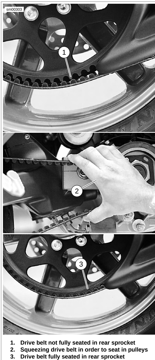
Figure 6-42. Seating Drive Belt Into Pulley Teeth
