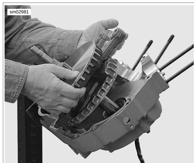
Figure 6-54. Removing Flywheels from Left Crankcase
