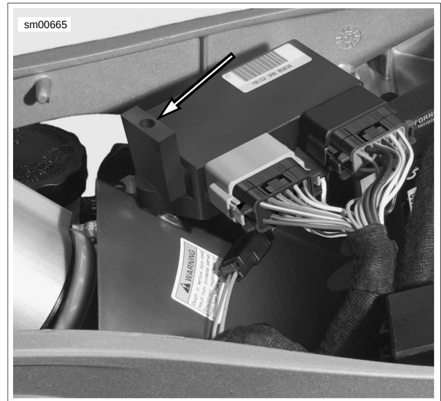
Figure 2-174. ECM Fastener with Captured Nut
