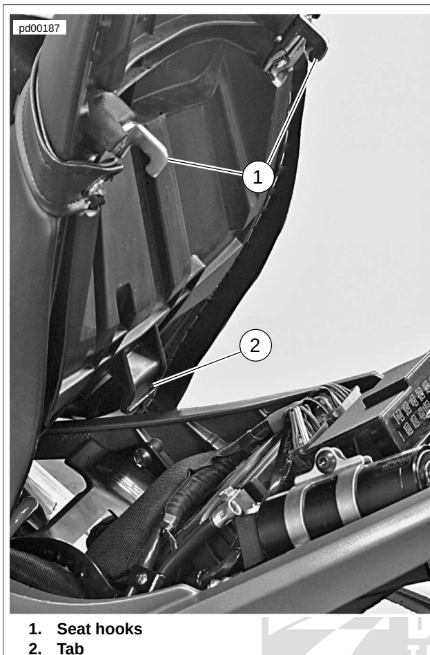
Figure 2-198. Fitting Seat Hooks to Frame Mounting Posts
