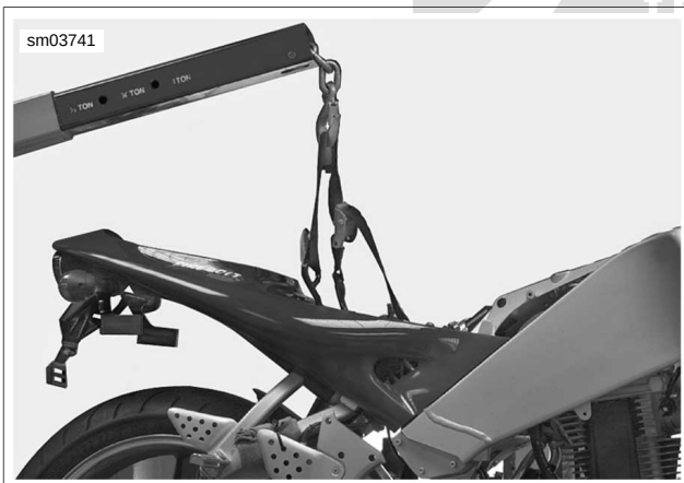
Figure 3-30. Supporting Vehicle for Disassembly
