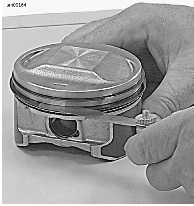
Figure 3-81. Measuring Ring Clearance in Groove
