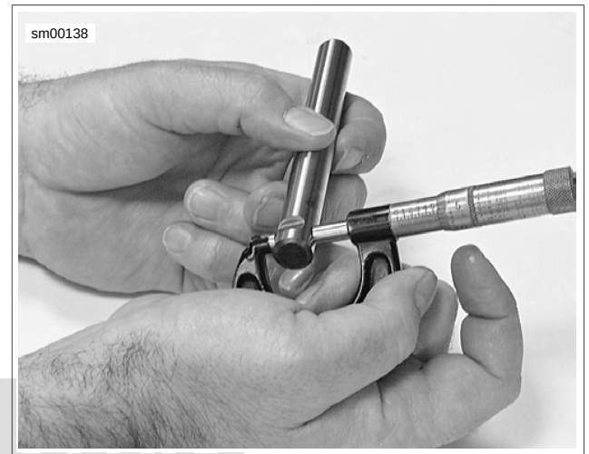
Figure 3-50. Measuring Rocker Arm Shaft Diameter (Rocker Cover Position)
