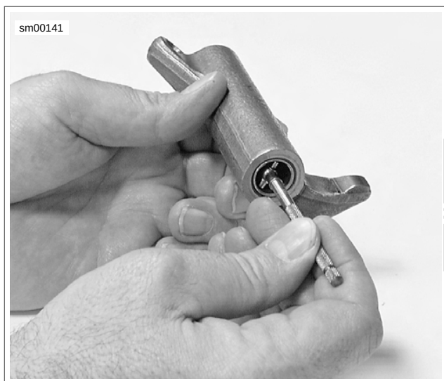
Figure 3-53. Measuring Rocker Arm Bushing Inner Diameter
