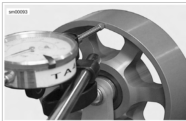
Figure 1-30. Measuring Lateral Side Play on Idler Pulley
