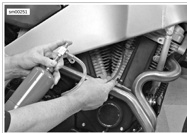
Figure 4-46. Checking for Intake Leak
