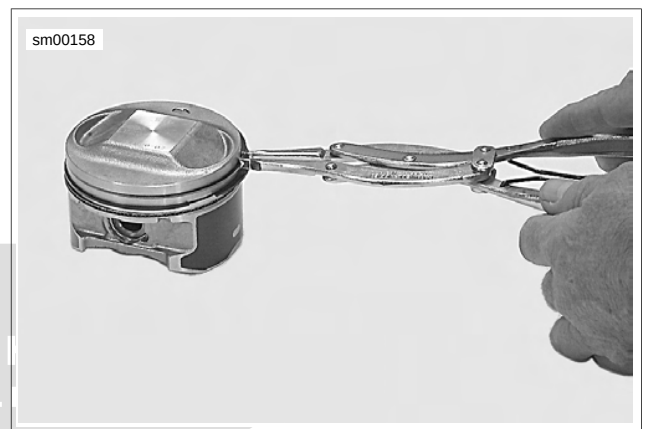
Figure 3-79. Installing Piston Rings Using Transmission Shaft Retaining Ring Pliers (Part No. J-5586-A)
