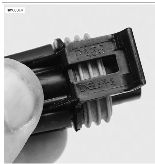
Figure A-12. Delphi Connector: Socket Housing Latch
