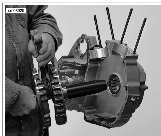
Figure 3-138. Installing Flywheel Assembly with CRANKSHAFT GUIDE
