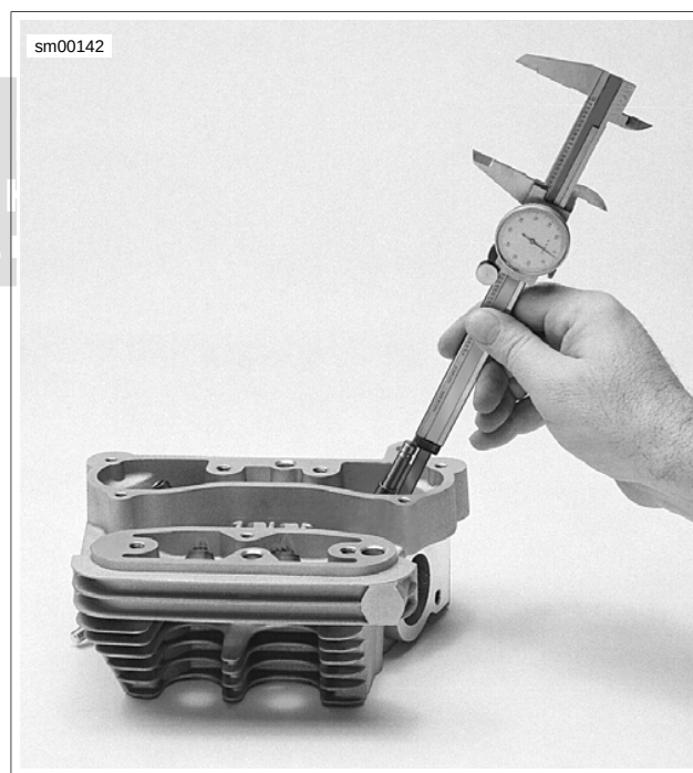
Figure 3-54. Measuring Valve Stem Protrusion
