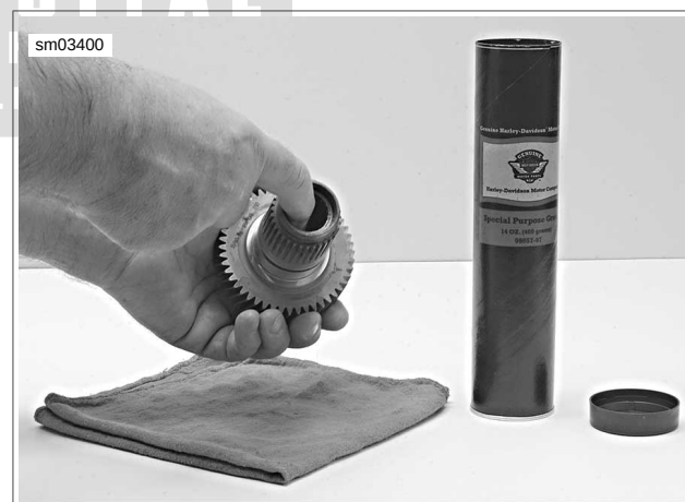
Figure 6-75. Lubricating Main Drive Gear Needle Bearing
