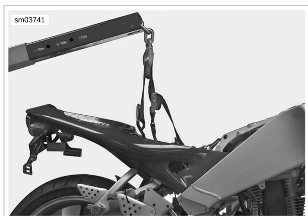
Figure 3-13. Supporting Vehicle for Disassembly
