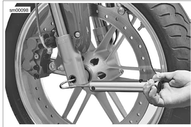
Figure 1-34. Measuring Steering Head Bearing Resistance (Typical)
