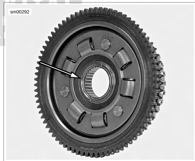
Figure 6-28. New Needle Bearing in Clutch Shell
