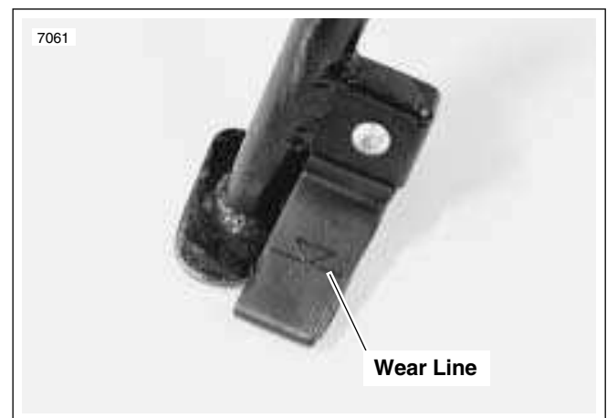
Figure 2-139. Side Stand Dragger Wear Limit
