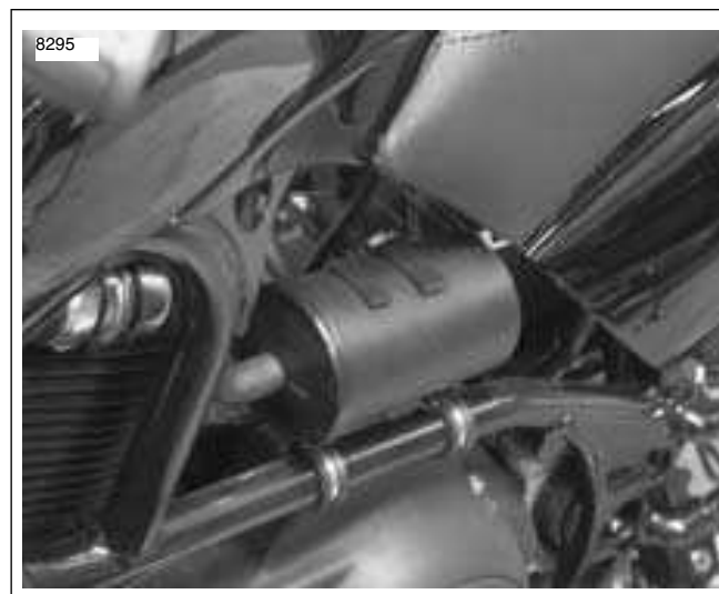
Figure 4-110. Carbon Canister Installation (Typical).
