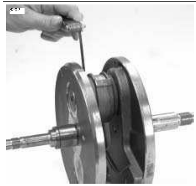
Figure 3-83. Checking Connecting Rod Side Play
