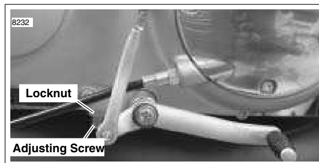
Figure 1-28. Measuring Primary Chain Adjustment
