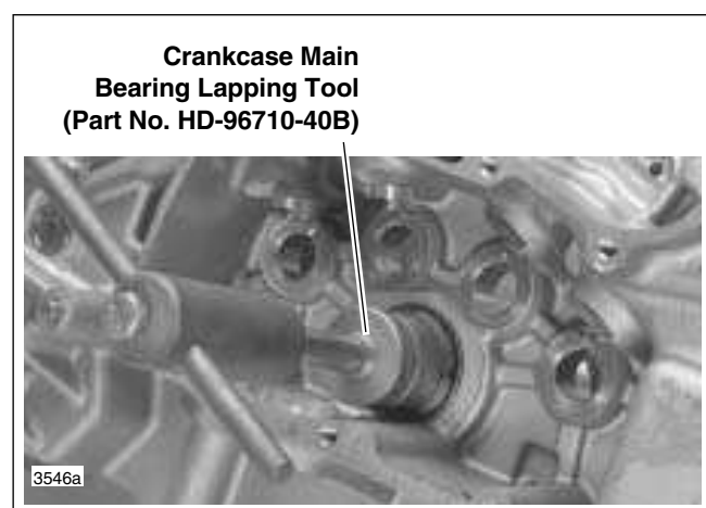
Figure 3-90. Lapping Pinion Shaft Main Bearing
