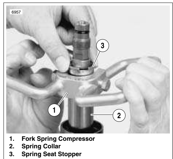
Figure 2-56. Front Fork Spring Compressor
