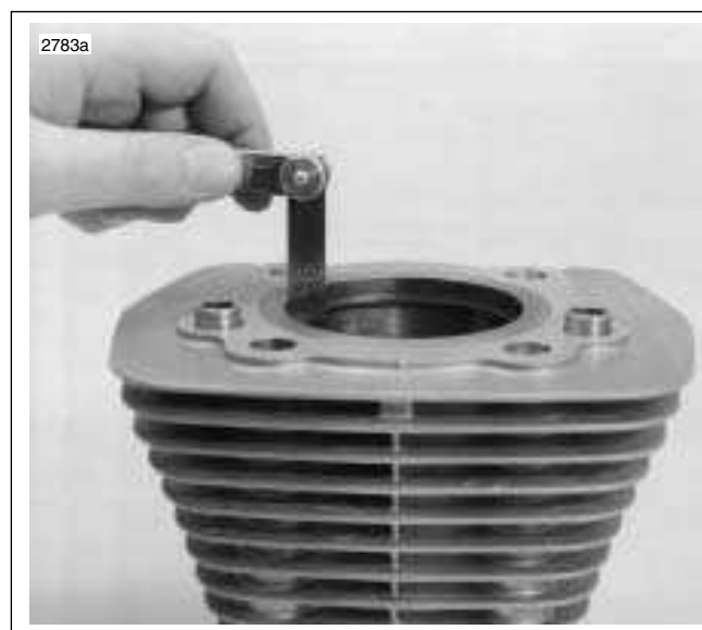
Figure 3-36. Measuring Ring End Gap
