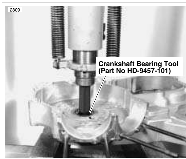
Figure 3-80. Sprocket Shaft Outer Race Removal
