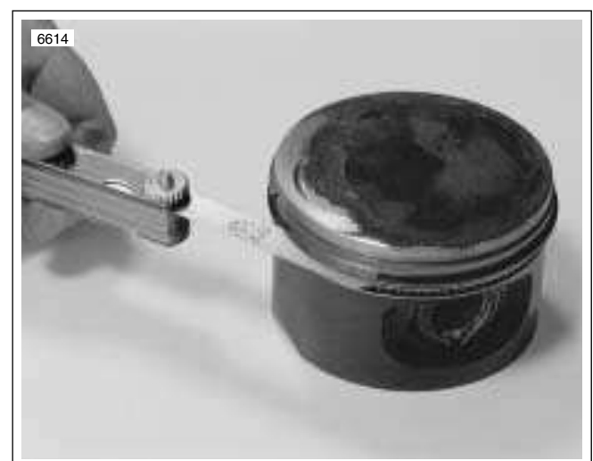
Figure 3-39. Measuring Ring Clearance in Groove
