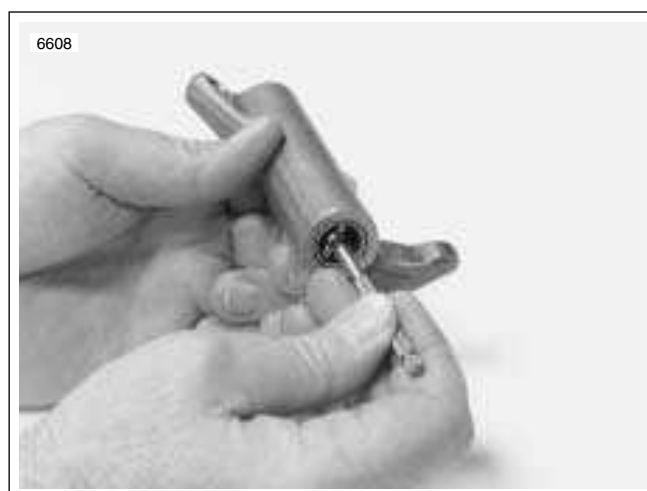
Figure 3-15. Measuring Rocker Arm Bushing Inner Diameter
