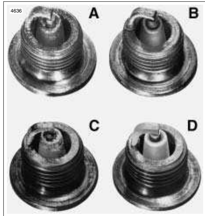
Figure 1-40. Typical Spark Plug Deposits
