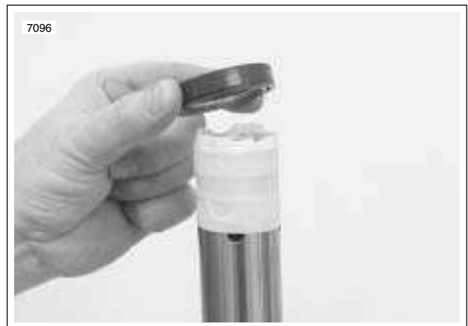
Figure 2-60. Slide Pipe Protection
