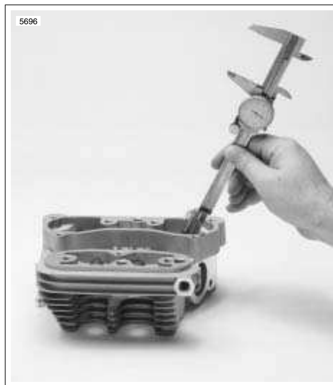
Figure 3-23. Measuring Valve Stem Protrusion
