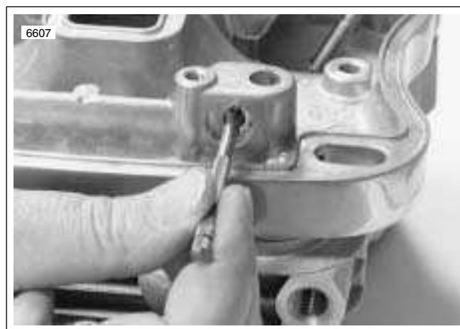
Figure 3-14. Measuring Rocker Arm Shaft Bore Diameter in Lower Rocker Cover
