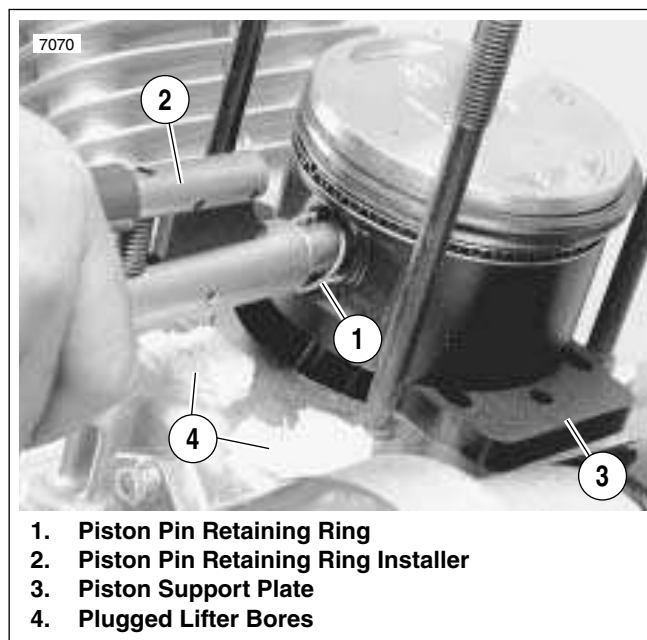
Figure 3-42. Installing Piston Retaining Rings
