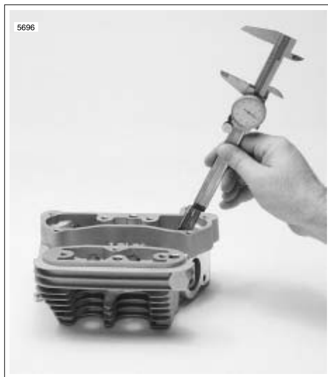
Figure 3-71. Measuring Valve Stem Protrusion
