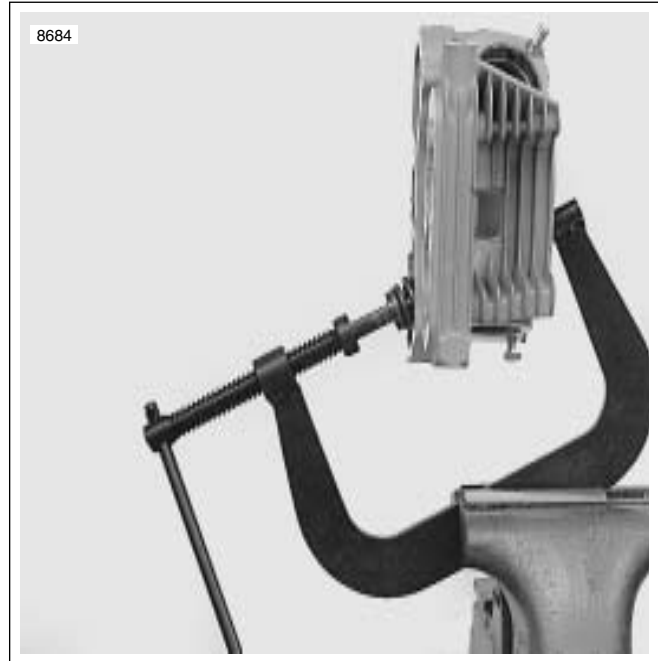
Figure 3-82. Valve Spring Compressor (Part No. HD-34736B)
