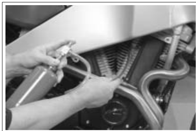
Figure 4-118. Checking for Intake Leak
