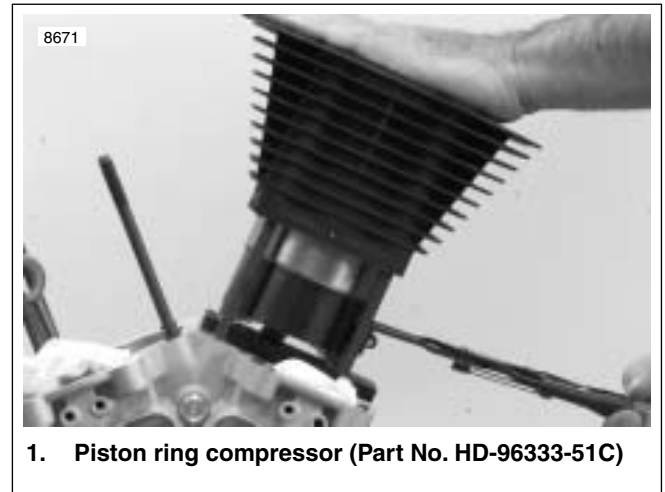
Figure 3-109. Compressing Piston Rings
