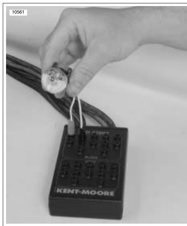
Figure 4-49. Testing Ignition Coil Connectors
