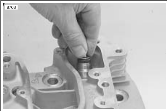
Figure 3-81. Valve Seal and Lower Collar Assembly Installation
