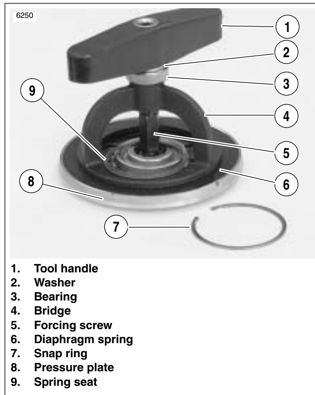
Figure 6-22. Pressure Plate Assembly
