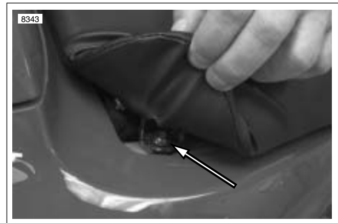
Figure 2-125. Accessing Rider Seat Screws
