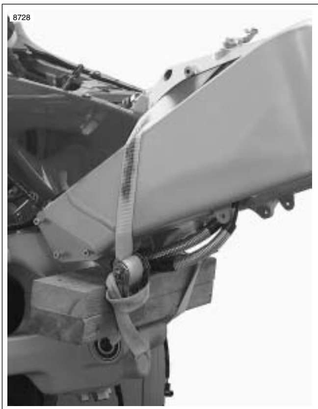
Figure 3-32. Securing Vehicle for Relocation
