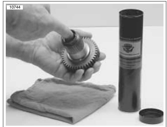
Figure 6-74. Lubricating Main Drive Gear Needle Bearings
