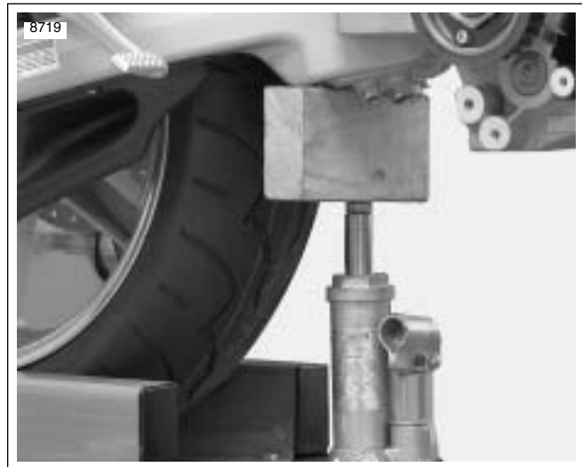
Figure 3-26. Supporting the Swingarm
