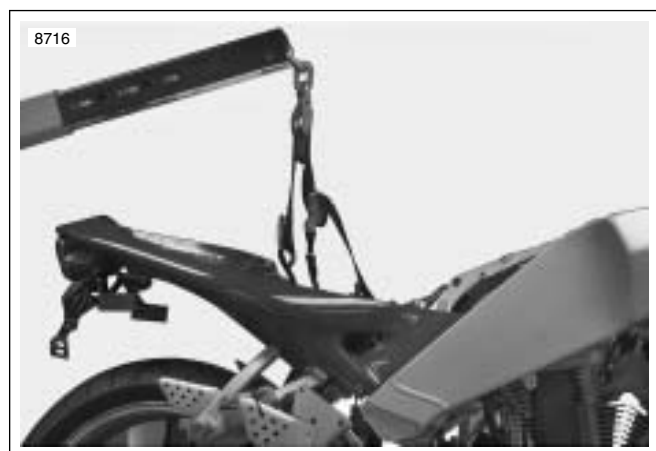
Figure 3-41. Supporting Vehicle for Assembly
