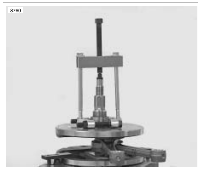
Figure 3-138. Removing Sprocket Shaft Inner Bearing Race
