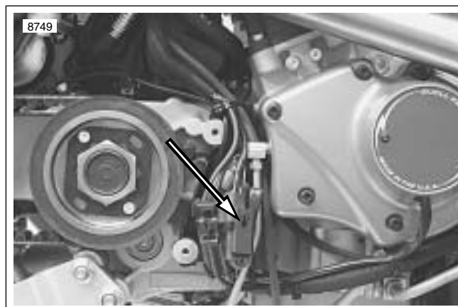
Figure 4-65. Cam Position Sensor Connector [14] (stator connector disconnected)
