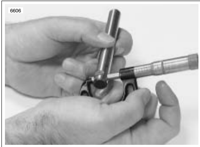
Figure 3-67. Measuring Rocker Arm Shaft Diameter (Rocker Cover Position)
