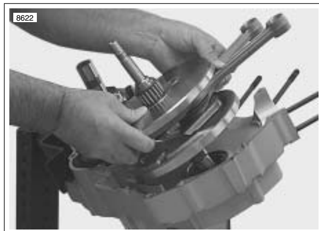
Figure 3-136. Removing Flywheels from Left Crankcase
