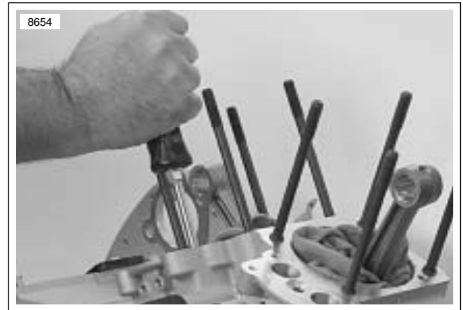
Figure 3-132. Checking Cam Gear End Play
