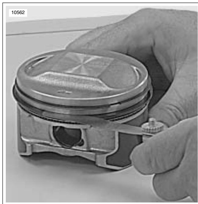
Figure 3-99. Measuring Ring Clearance in Groove
