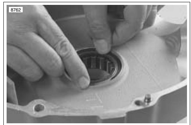
Figure 3-140. Removing Sprocket Shaft Bearing Retaining Ring
