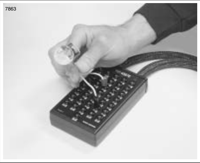
Figure 4-20. Ignition Coil Circuit Test
