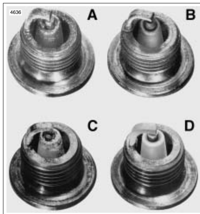
Figure 1-36. Typical Spark Plug Deposits
