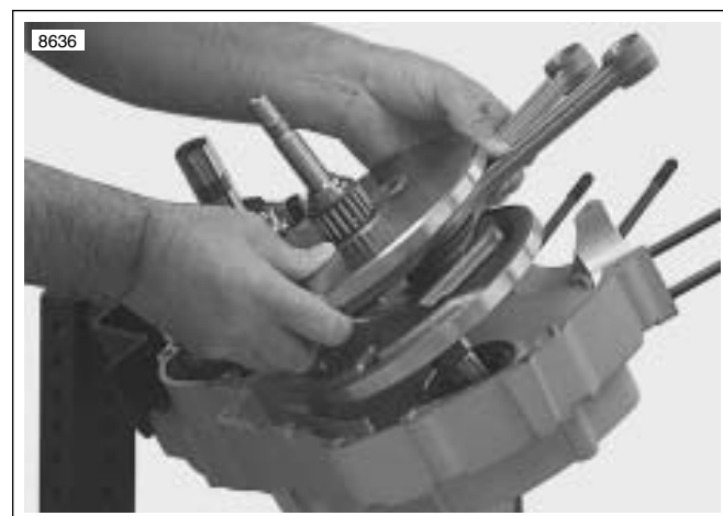
Figure 6-56. Removing Flywheels from Left Case Half
