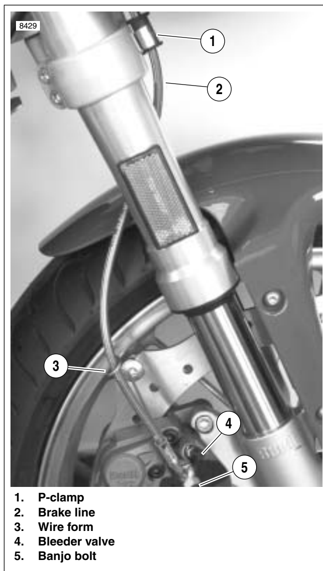
Figure 2-43. Front Brake Line
