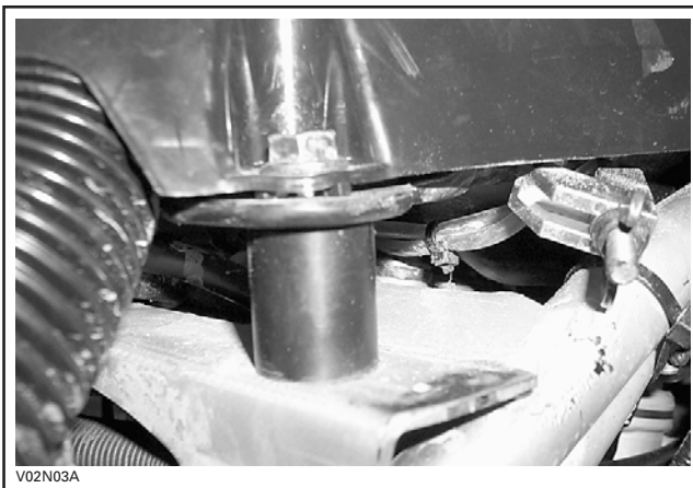
HOSE PINCHER INSTALLED ON FUEL TANK VENT LINE
