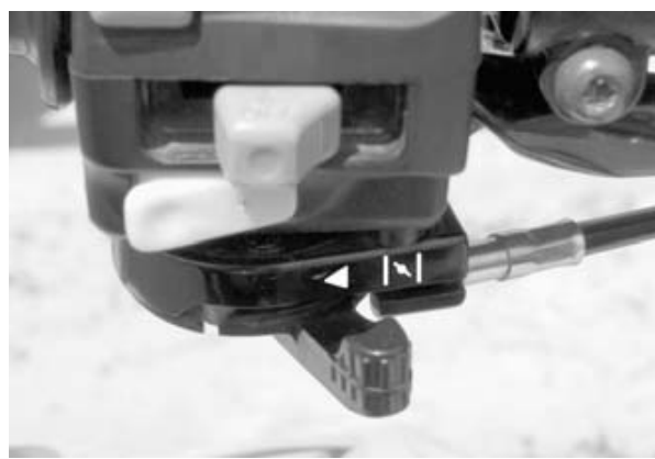
TYPICAL — CHOKE LEVER IN THE OFF POSITION
