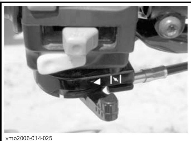
CHOKE LEVER IN THE OFF POSITION
