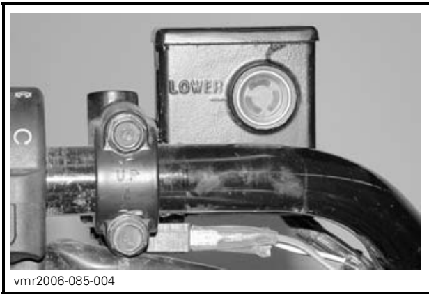
vmr2006-085-004 TYPICAL — LH REAR BRAKE FLUID RESERVOIR
