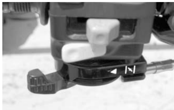
TYPICAL — CHOKE LEVER IN THE FULL CHOKE POSITION
