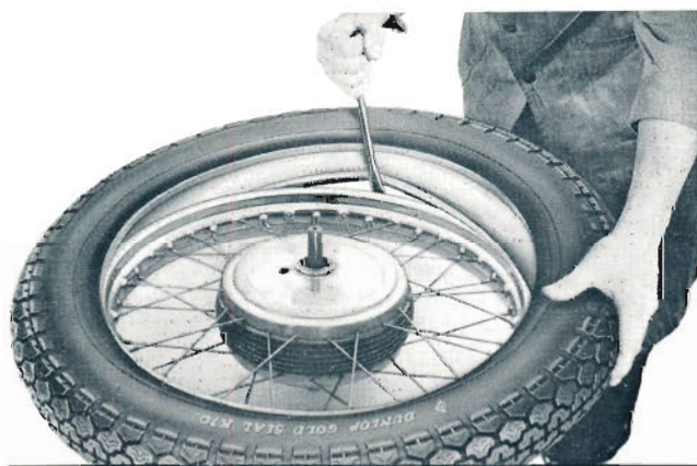
FIG. F.28. Completing the fitting of the first bead.
