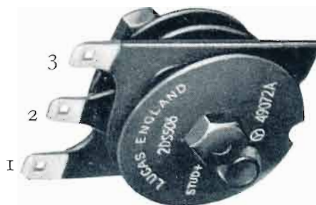
FIG. G.5. The rectifier showing terminal connections.
