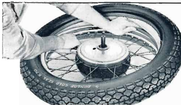
FIG. F.19. Fitting the first bead.
