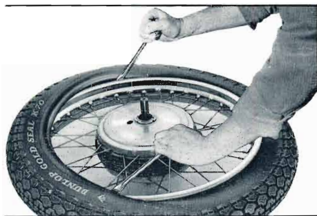
FIG. F.15. Removing the first bead.
