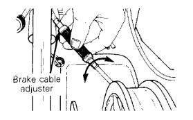
WARNING: Whenever the brake is readjusted, the brake light switch operation must also be checked and adjusted as needed.
