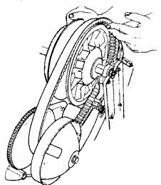
5. Lift the countershaft upward approx. 50 mm (2 in.) and slip the belt between the shaft and the bearing cage to remove completely.
