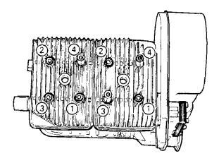
Following sequence above shown, torque engine head nuts twice.
