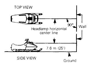
With the suspension correctly adjusted, the rider seated on the vehicle and the high beam ON check that the center of high intensity zone of high beam is 50 mm (2") below horizontal line of head-lamp height.
