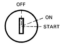
Key operated, 3 position switch. To start engine, turn key fully clockwise to START position and hold. Return key to ON position immediately when engine has started. To stop engine, turn key counter-clockwise to OFF position.
