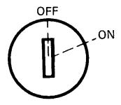
Key operated, 2 position switch. To start engine, first turn key clockwise to ON position. To stop engine, turn key counter-clockwise to OFF position.
