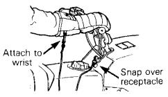
If emergency engine "**shut off**" is required, completely pull cap from safety switch and engine power will be automatically shut "off".
