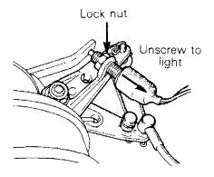
Tighten the brake switch lock nut and recheck brake light operation.
