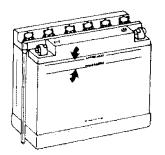
If necessary add distilled water. Battery connections must also be free of corrosion. If cleaning is necessary remove corrosion using a stiff brush then clean with a solution of baking soda and water. Rinse and dry well. CAUTION: Do not allow cleaning solution to enter battery. It will destroy the chemical properties of the electrolyte.
