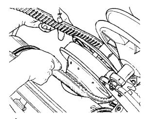
WARNING: After drive belt installation, always check that the brake disc is correctly installed between the brake pads and that the brake is well adjusted. Check brake light operation.
