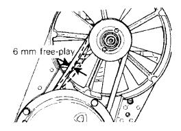
If belt seems damaged or if tension is incorrect, contact your dealer immediately.
