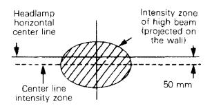
To adjust, remove the four caps, turn upper or lower adjusting screws to obtain desired beam position.
