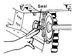
**Slide Suspension** Grease idler wheels at grease fittings.
