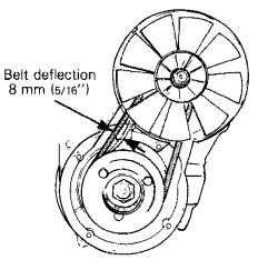
If the belt seems damaged or if tension is incorrect, contact your dealer immediately.
