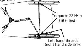
CAUTION: Do not overtighten the left hand threaded ball joint jam nut.
