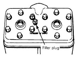
Refill tank until coolant overfills at filler hole.
