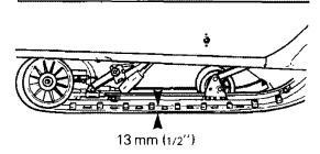
CAUTION: Too much tension will result in power loss and excessive stresses on suspension components.
