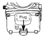
Re-install plug and connect fuel line. Check all fuel lines, replace if necessary.
